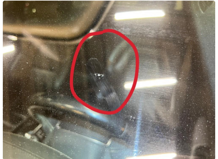
1.2 Steinsprut i synsfelt
