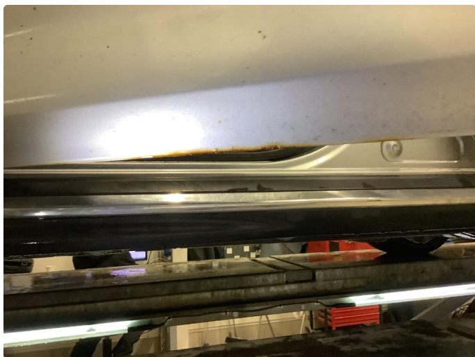
1.2 Rust i fals
