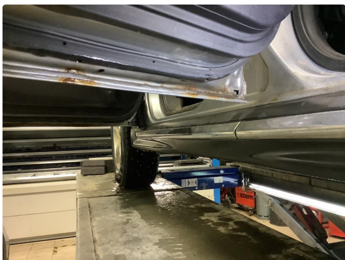
1.2 Rust i fals
