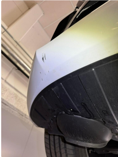
1.2 Noe skrubbskader underkant frontfanger.
