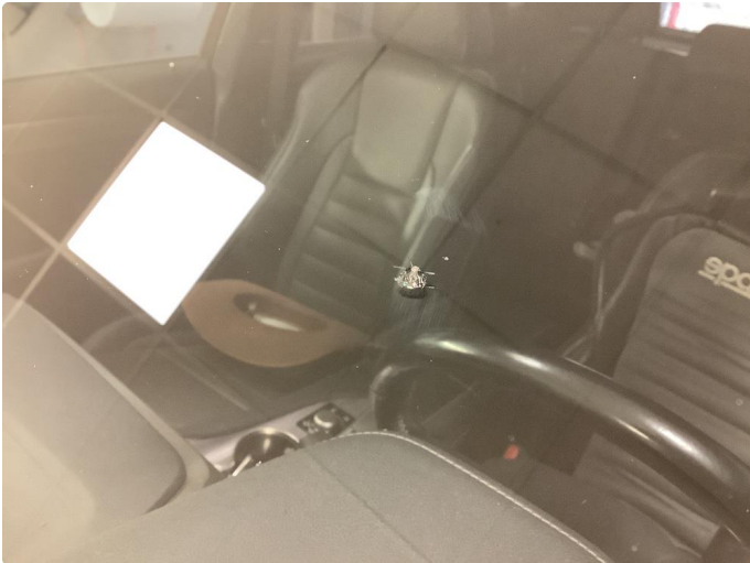
1.1 Steinsprut i synsfelt
