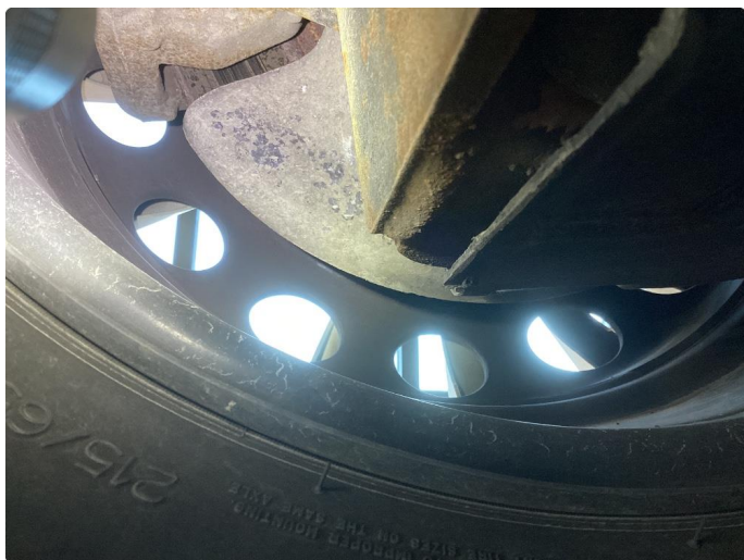
2.1 Mer enn 25% rust
