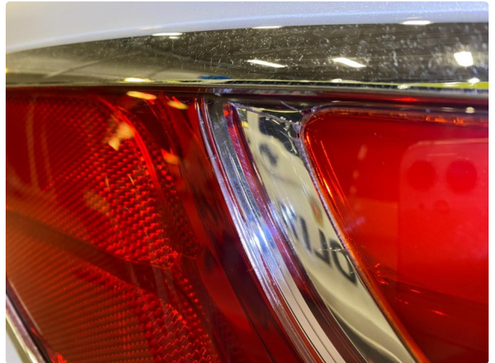
2.1 Krakelering i plast
