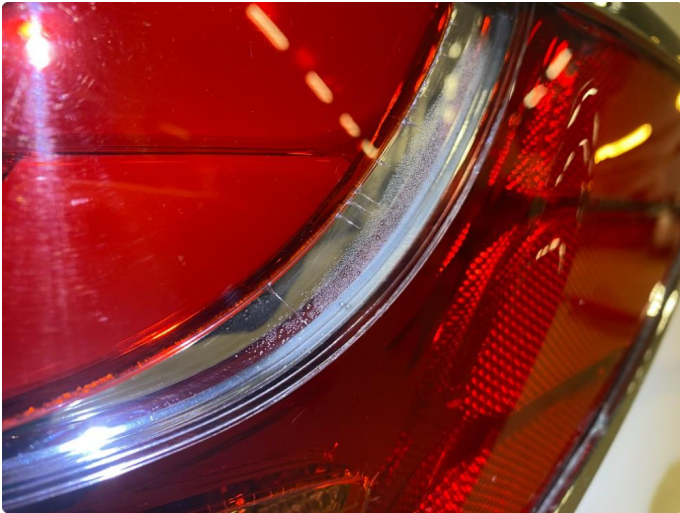
2.1 Krakelering i plast
