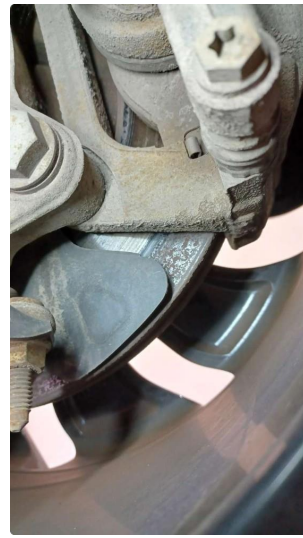
2.1 Mer enn 25% rust
