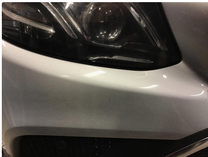
1.7 Noe steinsprut i front
