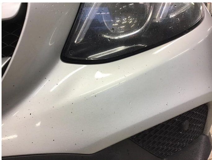
1.7 Noe steinsprut i front
