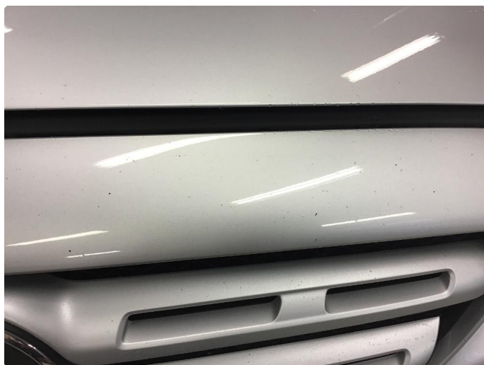
1.7 Noe steinsprut i front
