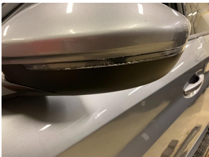
2.1 Krakelering i plast
