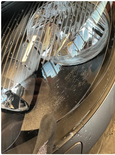
2.1 Krakelering i plast
