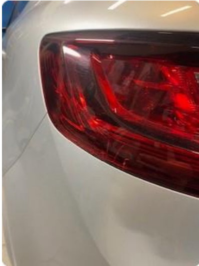
1.1 Defekt / sprukket glass
