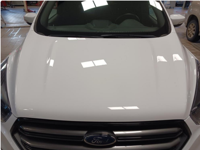
1.1 Panser lakeres pga steinsprut
