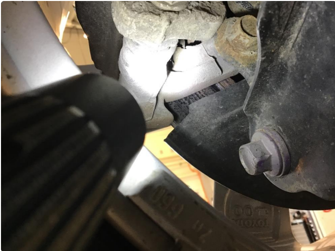
1.1 Mer enn 25% rust
