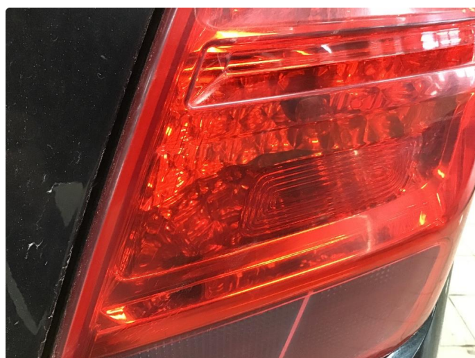
2.1 Krakelering i plast
