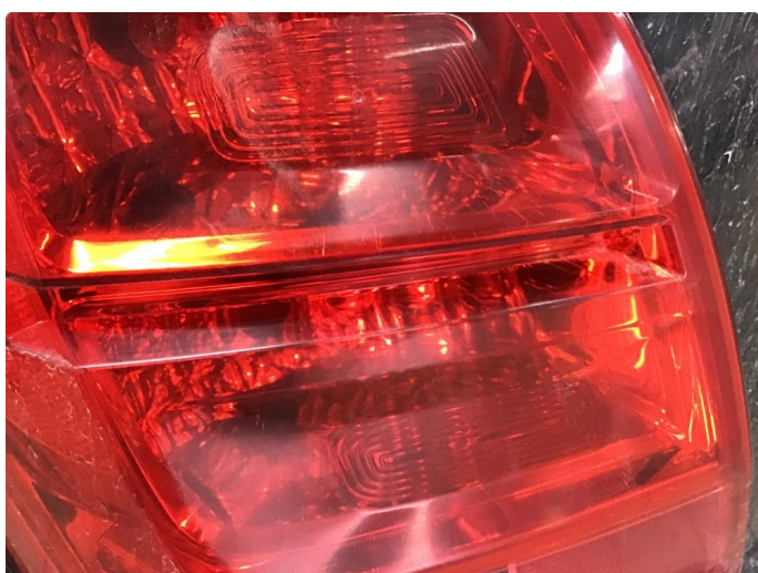
2.1 Krakelering i plast
