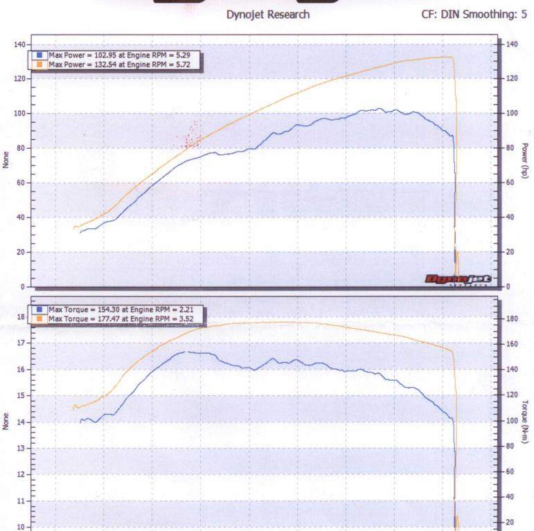
4,0 4,5 Engine RPM (rpmx1000)
