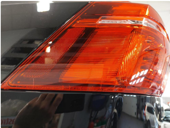
2.1 Krakelering i plast
