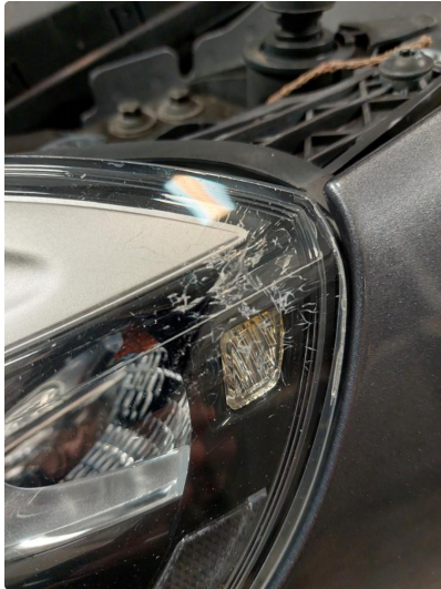
1.1 Krakelering i plast
