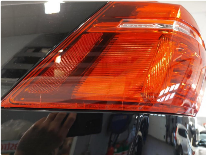
2.1 Krakelering i plast
