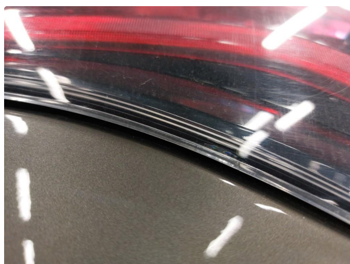
2.1 Krakelering i plast
