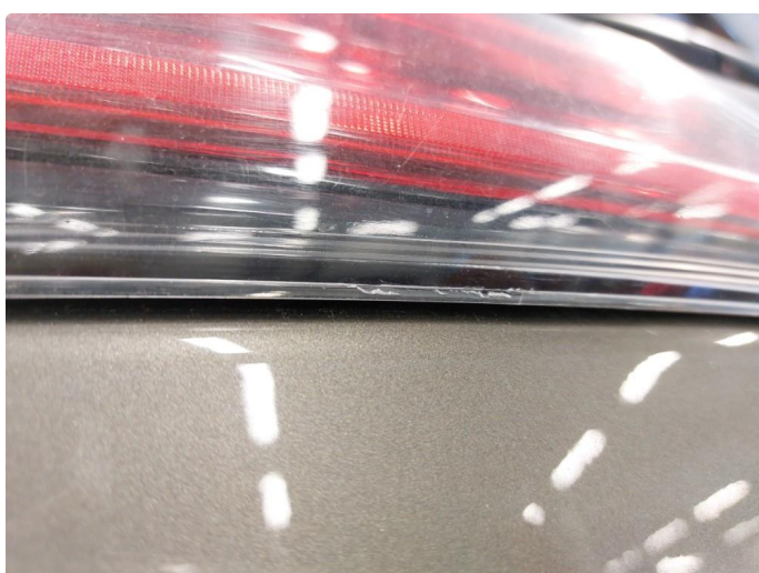
2.1 Krakelering i plast
