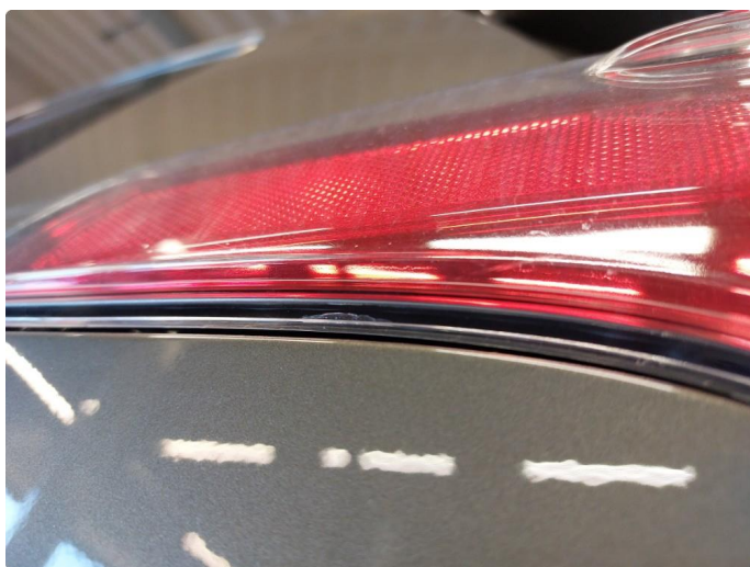
2.1 Krakelering i plast
