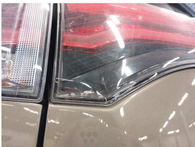
2.1 Krakelering i plast
