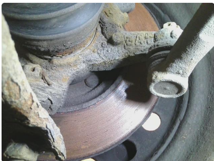
5.1 Mer enn 25% rust
