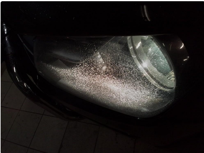
2.1 Krakelering i plast
