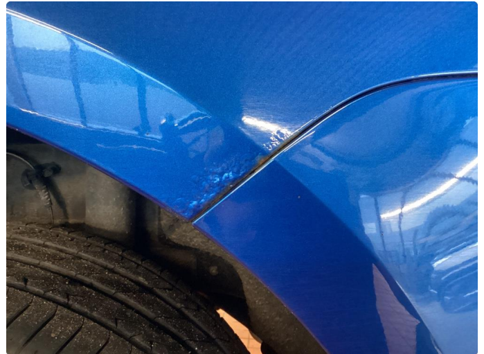
1.1 Rust under lakken
