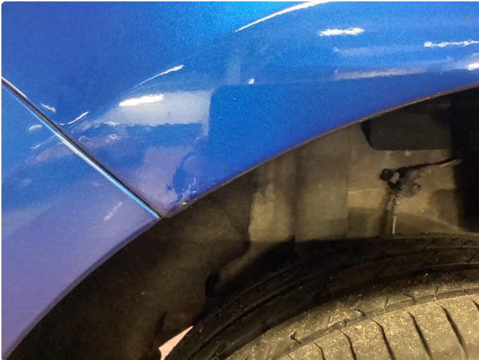
1.1 Rust under lakken
