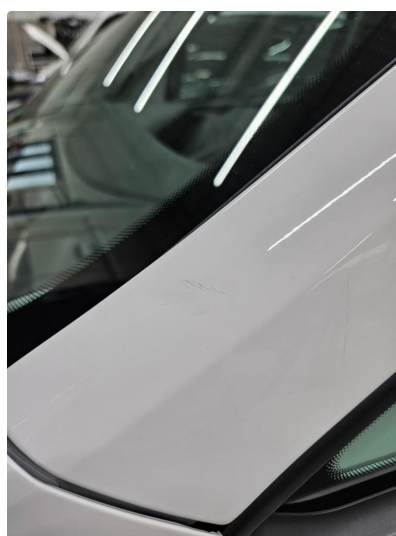
1.3 Liten bulk, A-stolpe v.side, blitt penslet m/lakk
