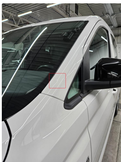
1.3 Liten bulk, A-stolpe v.side, blitt penslet m/lakk
