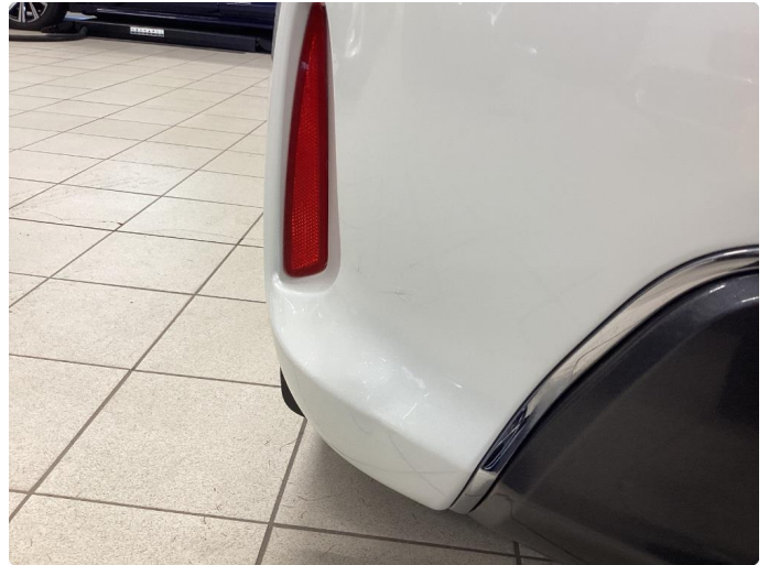
1.2 Liten bulk/sprekk i bakfanger
