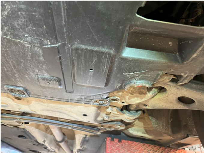
1.1 Sprekk i plastplate under bil
